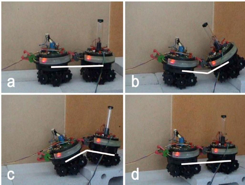
Figure 5: Example of a task that two s-bots can perform together, but not in isolation. Using the rigid connection between them, (a) one s-bot is helped to pass the step (b). As soon as the first s-bot has passed, it helps the second to pass the step too (c and d).
