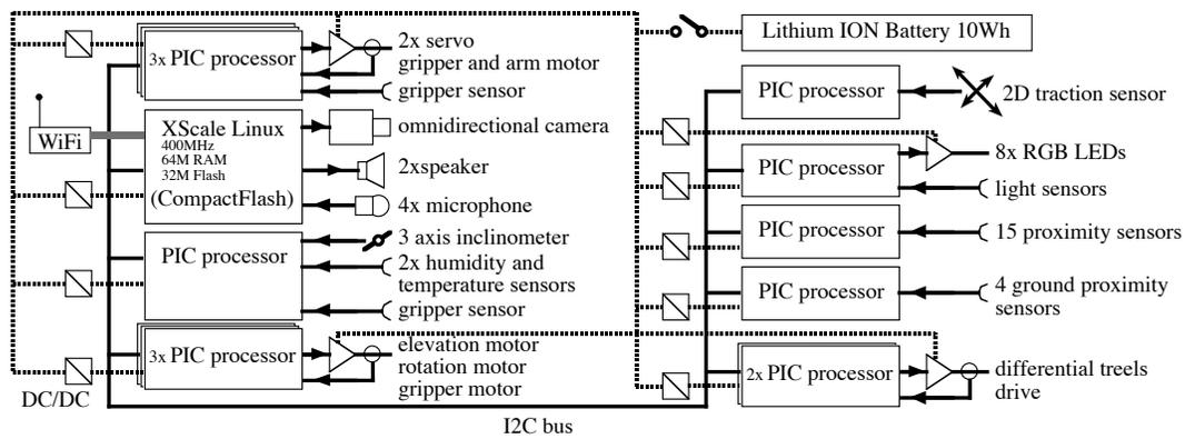
Figure 4: Schematic structure of the s-bot electronics. Fourteen processors distributed all around the robot body manage all the sensor and actuator devices.
